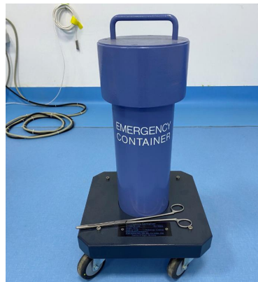
备用储源铅罐
